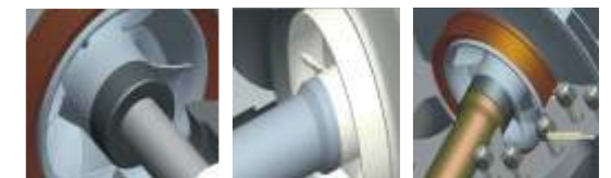
Conventional method of impeller & nut arrangement
