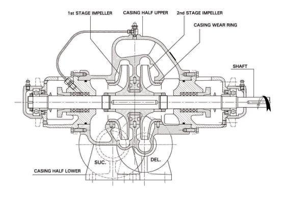
DSM (Non Thru Bore) Pump - Typical Drawing
