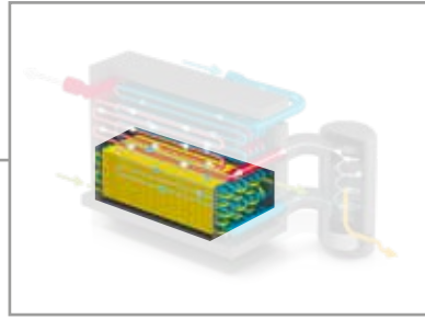
Air/refrigerant heat exchanger with thermal mass (yellow area)
