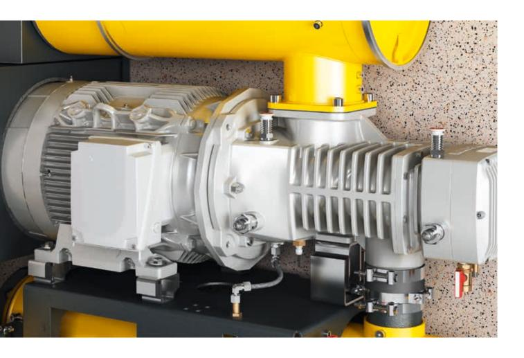
In CBS, DBS and EBS series rotary screw blowers, power is transferred from the motor to the blower airend via integrated gearing. This has proven to be the best solution for the prevailing speeds in this performance and size class when it comes to efficiency, reliability and durability. In the case of HBS series blowers, power is transferred directly, without losses, via a coupling. These design concepts are the result of extensive research at KAESER's Research and Development Centres.
