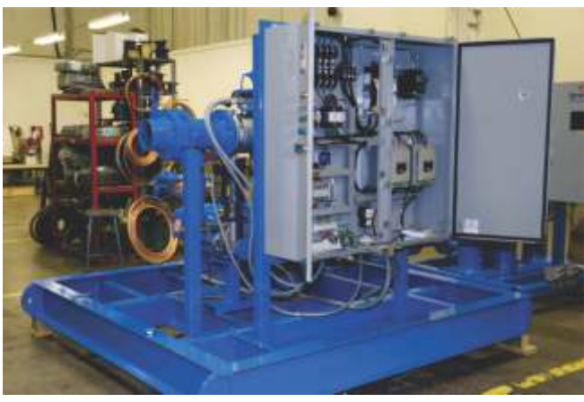
Skid mounted VFD panel
